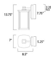
height from center of outlet to top of the foture
