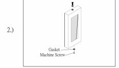
Step.2: Re-install fixture (B) to back-plate (A) and tighten worm screws (C) with rubber gasket (D) provided so that fixture meets the wall. Caulk around back plate where it meets the wall using outdoor silicone sealant.
