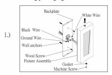
Step.1: Remove backplate (A) from fixture (B) and install it to electrical box. Wire fixture to wires in outlet box. Copper wire is for ground.
